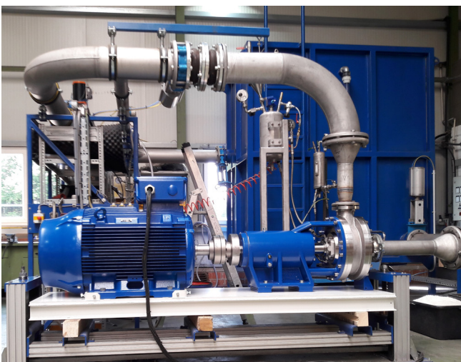
GORAMILL ® 33, 160 kW on the test rig: development and analysis – a must
