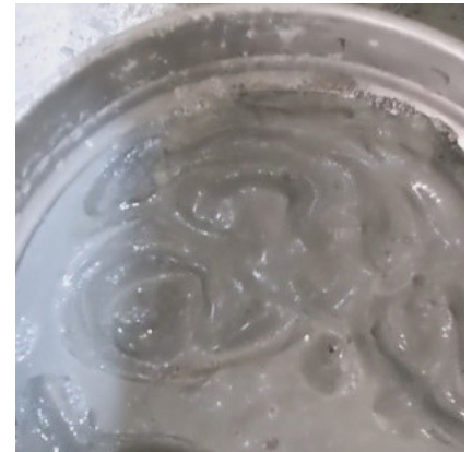
up to fine pudding-like slurry (d90 ~ 100 \mu )
